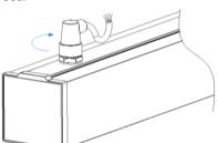
(5) Connect the lamp input line in outlet box according to the color mark corresponding to the city electricity and dimming signal line, strain relief device needs to be used before cord entry the oulet box during installation
